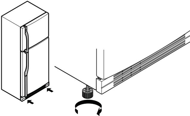
4. Open both doors again and check to make sure that they close easily. If not, tilt the refrigerator slightly more to the rear by turning both leveling screws clockwise. It may take several more turns, and you should turn both leveling screws the same amount.
